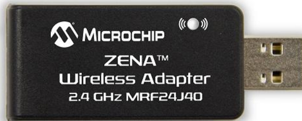
ZENA™ Wireless Adapter – 2.4 GHz MRF24J40 (Part # AC182015-1)
