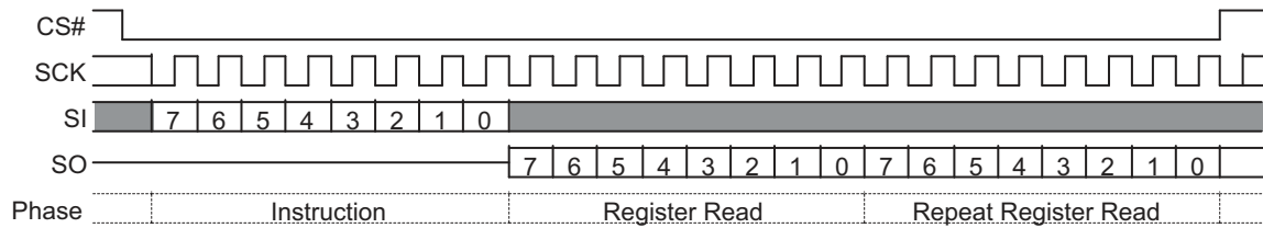
Figure 9.23 DLP Read (DLPRD) Command Sequence
