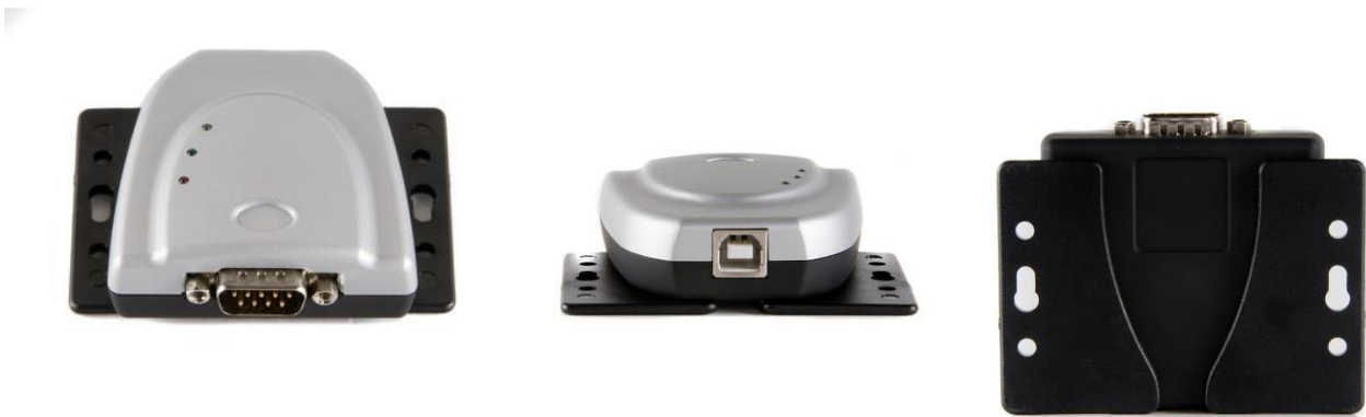
Figure 2.1 - USB2-F-5001 with UniClip Brackets
