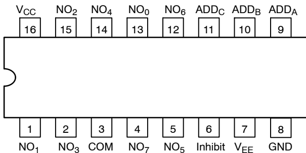
Figure 1. Pin Connection (Top View)
