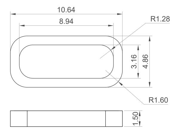
Recommended Waterproof Gasket Spec Material: Silicone Rubber, Shore Hardness 60A, Colour: Black Used with: USB4715
