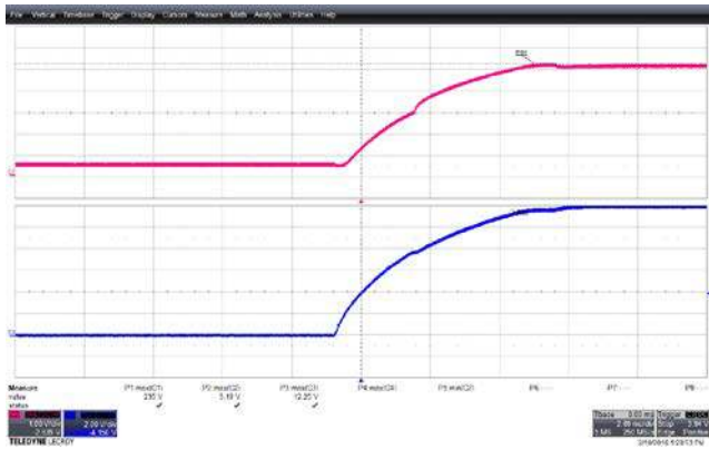
Figure 32 – Output Voltage Waveforms. 85 VAC Input. Upper: 5 V, 1 V / div. Lower: 12 V, 2 V / div, 2 ms / div.
