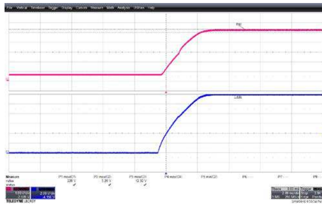
Figure 34 – Output Voltage Waveforms. 85 VAC Input. Upper: 5 V, 1 V / div. Lower: 12 V, 2 V / div., 2 ms / div.
