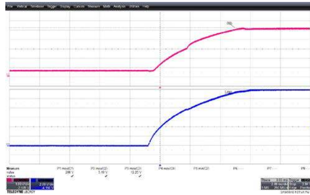
Figure 33 – Output Voltage Waveforms. 484 VAC Input. Upper: 5 V, 1 V / div. Lower: 12 V, 2 V / div., 2 ms / div.
