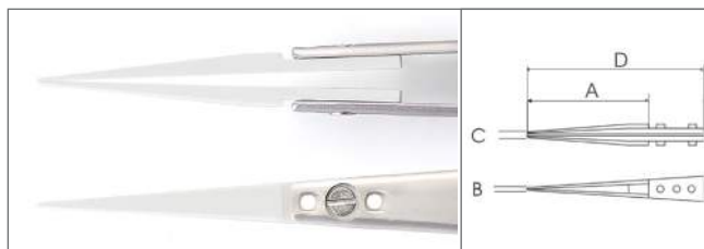
71MZ.SA A 1.18" 30 mm - B 0.028" 0.7 mm - C 0.05" 1.2 mm - D 1.8" 45 mm _ Replaceable tips set code: A71MZ
