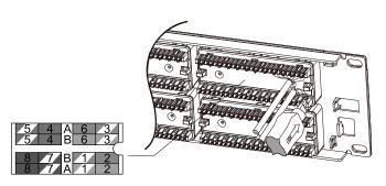
2. Punch down solid cable to each port until termination is completed.
