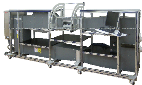
Fig. E: FDK Original Wind Tunnel
