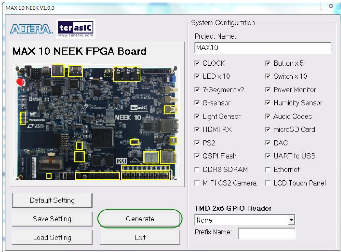
Figure 4-6 Generate Quartus Project
