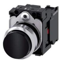
Pushbutton, 22 mm, round, metal, shiny, black, pushbutton, raised, momentary contact type, with holder, 1 NC, screw terminal
