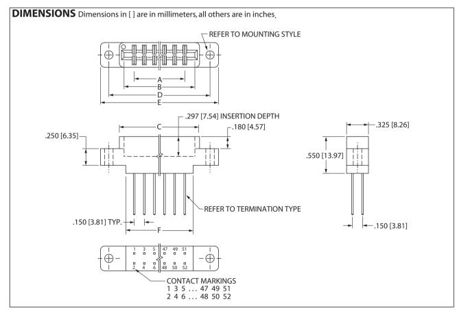
Tolerances on non-critical dimensions may very slightly due to shrinkage differential per insulator material; Consult factory.
