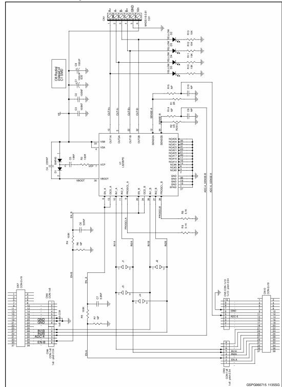
Figure 1: X-NUCLEO-IHM04A1 circuit schematic
