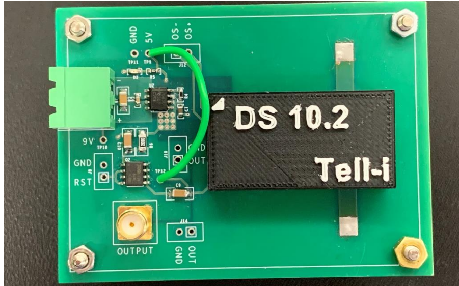
Figure 4: Demonstration of Reset (Testpoint 9 short to Testpoint 12)
