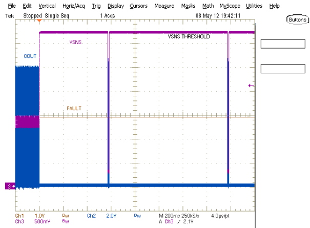
Figure 18 · VSNS Threshold No Fault
