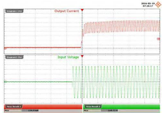
Figure 62 – 230 VAC, 48 V LED, Output Rise. Upper: I_{OUT} , 40 mA / div. Lower: V_{IN} , 100 V / div., 100 ms / div.
