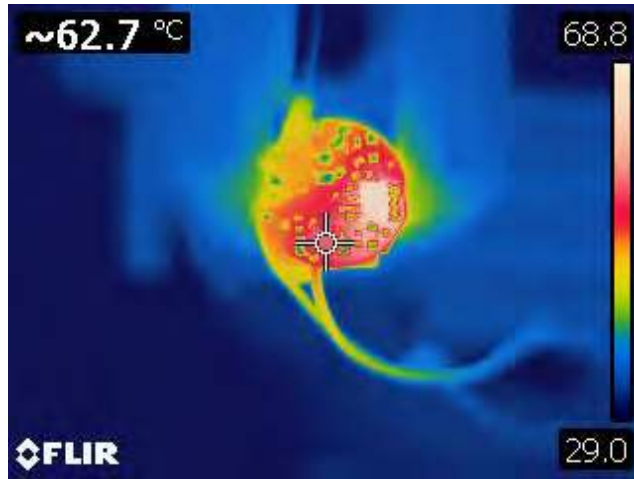
Figure 35 – 300 VAC, 48 V LED Load. Spot 1: Flywheel Diode (D1): 62.7 °C.
