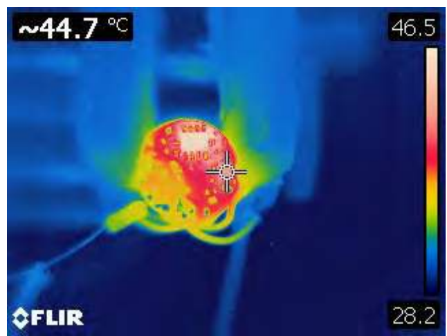
Figure 45 – 230 VAC, Output Short. Spot 1: Flywheel Diode (D1): 44.7 °C.
