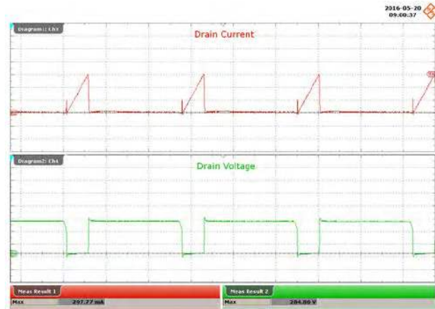
Figure 74 – 230 VAC, 48 V LED Load. Upper: I_{DRAIN} , 100 mA / div. Lower: V_{DRAIN} , 100 V / div., 5 \mu s / div.
