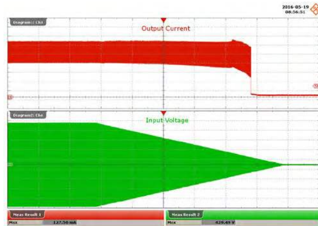
Figure 118 – Brown-out Test at 1 V / s. Ch1: I_{OUT} , 20 mA / div. Ch2: V_{IN} , 100 V / div. Time Scale: 50 s / div.
