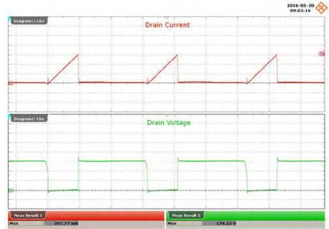
Figure 72 – 115 VAC, 48 V LED Load. Upper: I_{DRAIN} , 100 mA / div. Lower: V_{DRAIN} , 50 V / div., 5 \mu s / div.
