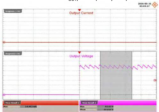
Figure 96 – 300 VAC, Open Load. Open Load Start-up. Upper: I_{OUT} , 40 mA / div. Lower: V_{OUT} , 10 V / div., 4 s / div.
