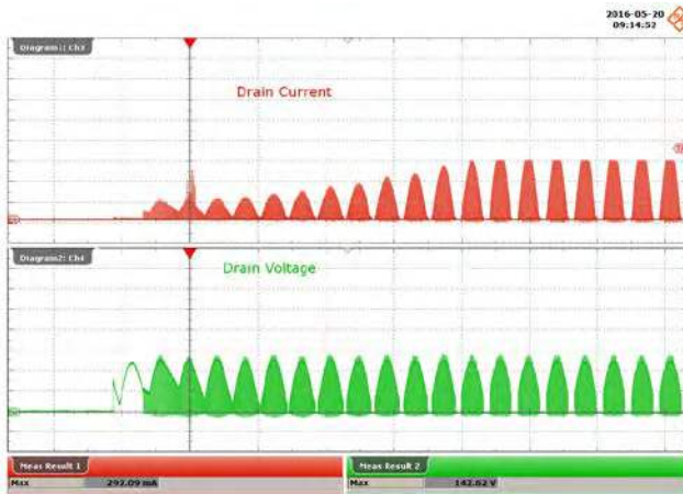
Figure 77 – 90 VAC, 48 V LED Load. Upper: I_{DRAIN} , 100 mA / div. Lower: V_{DRAIN} , 50 V / div., 20 ms / div.
