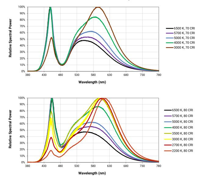
The following graphs are the result of a series of pulsed measurements at 1100 mA and T<sub>1</sub> = 85 °C.
