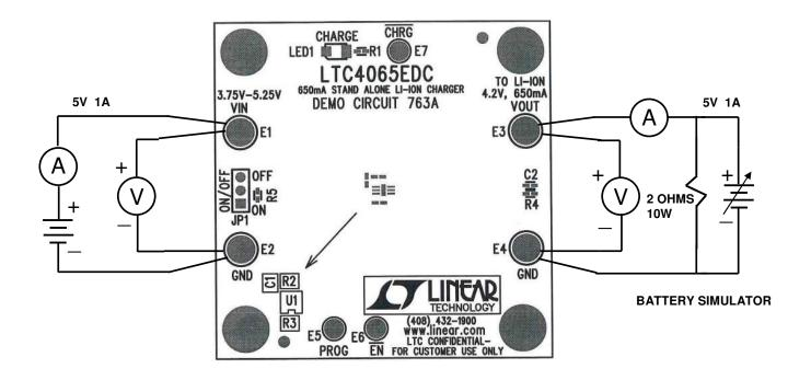
Figure 1. Proper Measurement Equipment Setup
