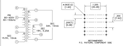
Application of the transformer allows for the leadwires between terminals 8&9 and 10&11 to solder bridge.
