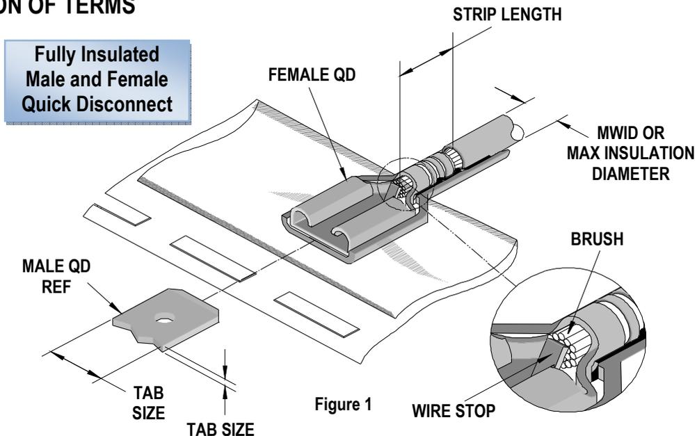
The following illustrations are a generic terminal representation and not an exact image of any terminal listed in the scope.
