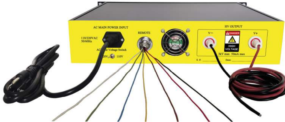
Figure 4. Back panel connection
