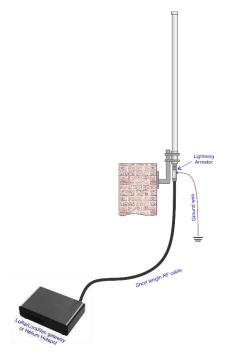
This is the simplest case and best option if the gateway is not far from the antenna, typically the RF cable length outdoors should be 2 meters or less, although cable length indoors may be larger.
