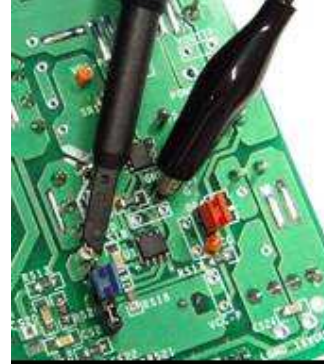
Fig. 4C Connecting O-scope probe to hook Gate drive test points.
