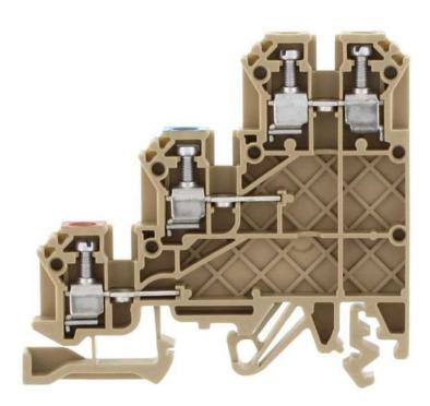
Three-level initiator terminal, Screw connection, Mounting type:Mounting rail TS 35/7.5 and TS 32, Rated cross-section: 2.5 mm², Width: 5 mm, Colour: Beige
