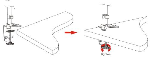
Turn the knob to make clamp fit to desk edge, then secure it tightly.
