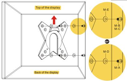
Choose appropriate screws and washers according to the type of your display, attach the VESA plate to the back of the display and tighten the screws using a Philips screwdriver.
