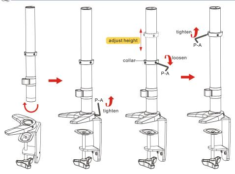
Insert the pole (B) into the desk clamp (C) and tighten the screws using 3mm Allen Key (P-A). To adjust monitor height, first loosen collar screws using 3mm Allen Key (P-A), then set the collar at a desired position and tighten the collar screws using 3mm Allen Key (P-A).
