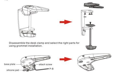
Re-install the base plate with the three retained screws, and then tighten securely using a 4mm Allen Key (P-B). Then attach silicone pad for each screw.
