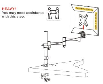
Lift your display and guide the screws into the mounting holes on the mount
