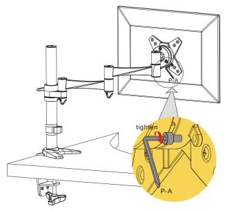
Attach the VESA plate to the mount with the retained screws from Step #2 (see page 3) and tighten them using a 3mm Allen Key (P-A).
