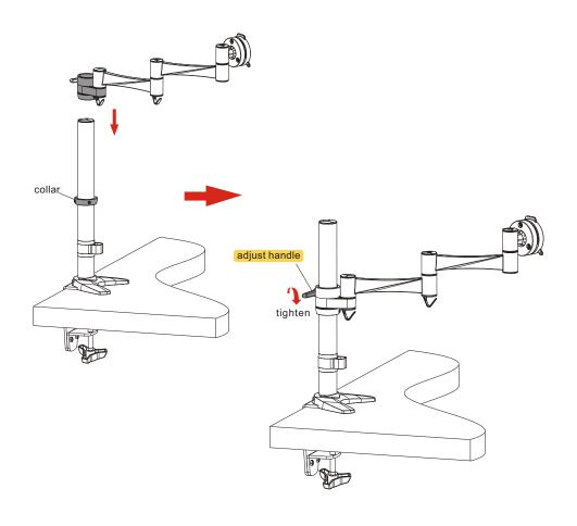
Insert the articulated arm assembly into the pole until it touches the collar. Then tighten the adjust handle.
