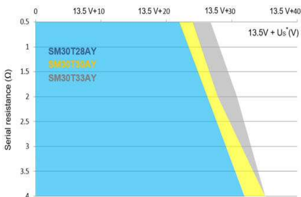
Figure 19. Load dump capability ( U_s^* = f(R_i) pulse 5b, U_s = 87\text{ V} , t_p = 400\text{ ms} )
