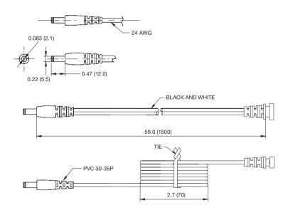
Wire type: VW-1 80°C 300 V L=1500 mm 2468, 18 AWG for 12 V output, 20 AWG for 15 V output, 22 AWG for 18 and 24 V output, 2C Black and White. Black - Negative, White - Positive
