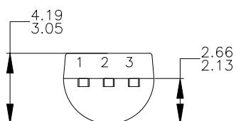
**Mechanical Dimensions** (Continued)**Package****Dimensions in millimeters****TO-92 Formed Lead For T&R and Ammo Packing**
