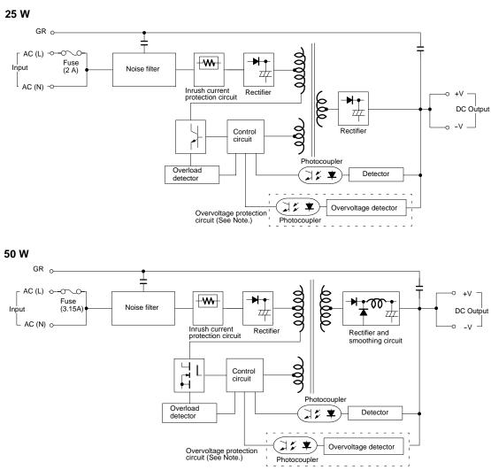
Note: Only the S8E1 with an output of 5 V incorporates an overvoltage protection circuit.
