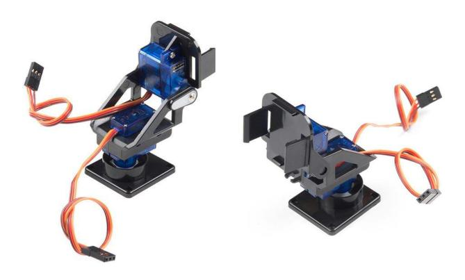
This is an easy-to-assemble pan/tilt bracket kit that utilizes servos to move on two axes fit for camera and helping-hand applications. This particular bracket kit is the same one we use in our SparkFun Raspberry Pi Zero W Camera Kit to create a remote camera system for your home or workplace.
