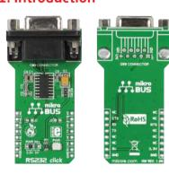
RS232 click<sup>™</sup> is a simple solution for adding RS232 serial communications to your design. The board features a standard RS232 DB9 port and a MAX3232 IC, along with a mikroBUS" host socket, three jumpers and a power indicator LED. RS232 click™ communicates with the target board through mikroBUS™ RX (RXD), TX (TXD), CS (RTS), and INT (CTS) lines. RS232 click™ is designed to use either a 3.3V or 5V power supply.
