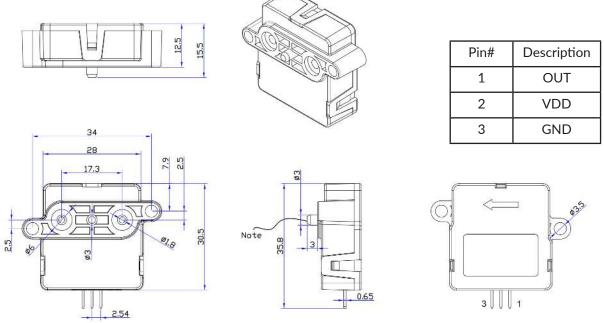
Note: The positioning hole on the manifold that receives the post shall have a diameter between 3.2 and 3.3mm, and a depth greater than 3.3mm. Contact Posifa for sensor CAD model.
