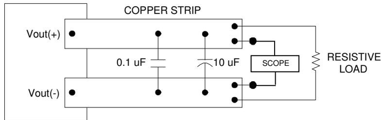
Note: Use a 0.1 $\mu$ F X7R ceramic capacitor and a 10 $\mu$ F @ 100V low ESR electrolytic capacitor. Scope measurement should be made using a BNC socket. Position the load 3 in. [76mm] from module.
