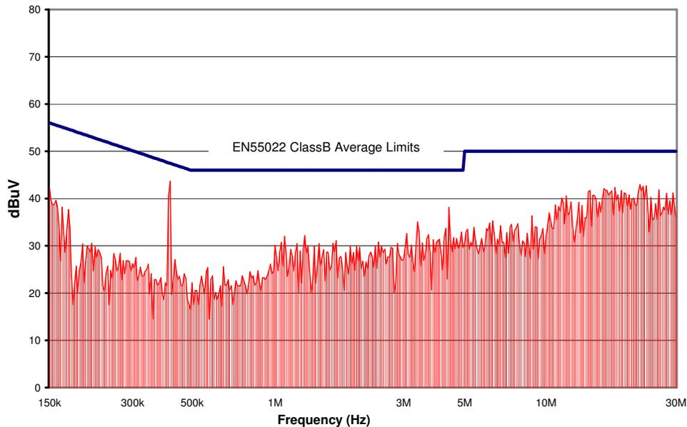
Figure 18. CPE2U36 Conducted Emissions using above specified input filter, Vin = 48V, Full Resistive Load
