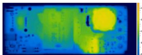
Thermal Image of module @ 48Vin, 200LFM & 55C
