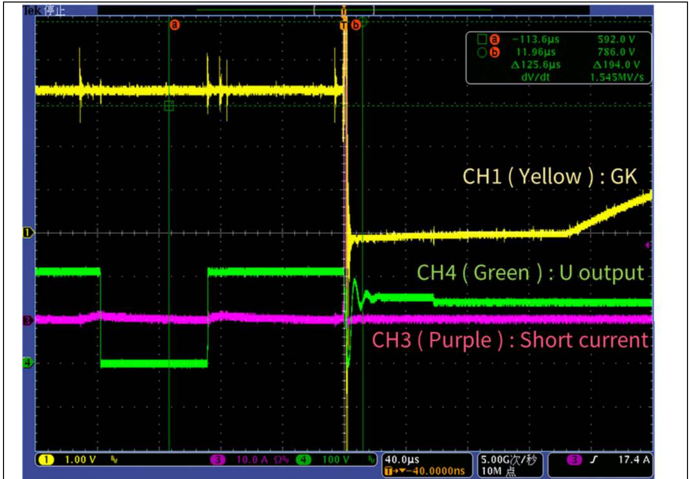
Figure 25 GK and U phase current and voltage waveform in short output on J2
