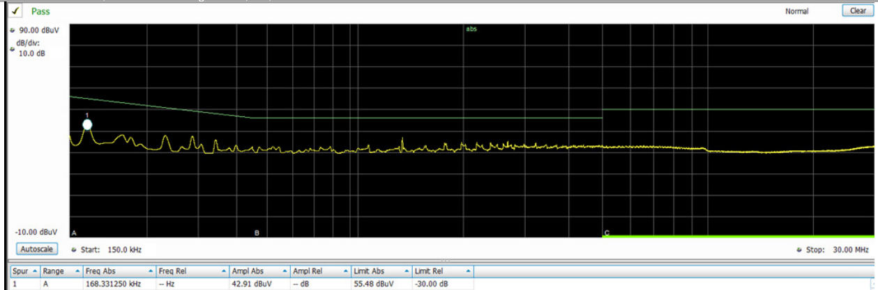
EMI; Conducted CISPR 22; Peak vs. Average Limit; L2/Neutral; 100Vac 24Vdc @ 25A dc
