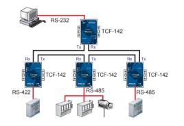
developed by Moxa RS-485 data direction automatically, making it unnecessary to use the
