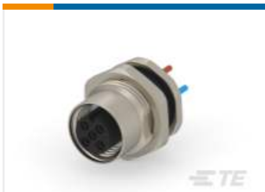
TE Part #T4171110003-001 M12,REAR MOUNTING,FEMALE,A,3P, 0.2M WIRE
