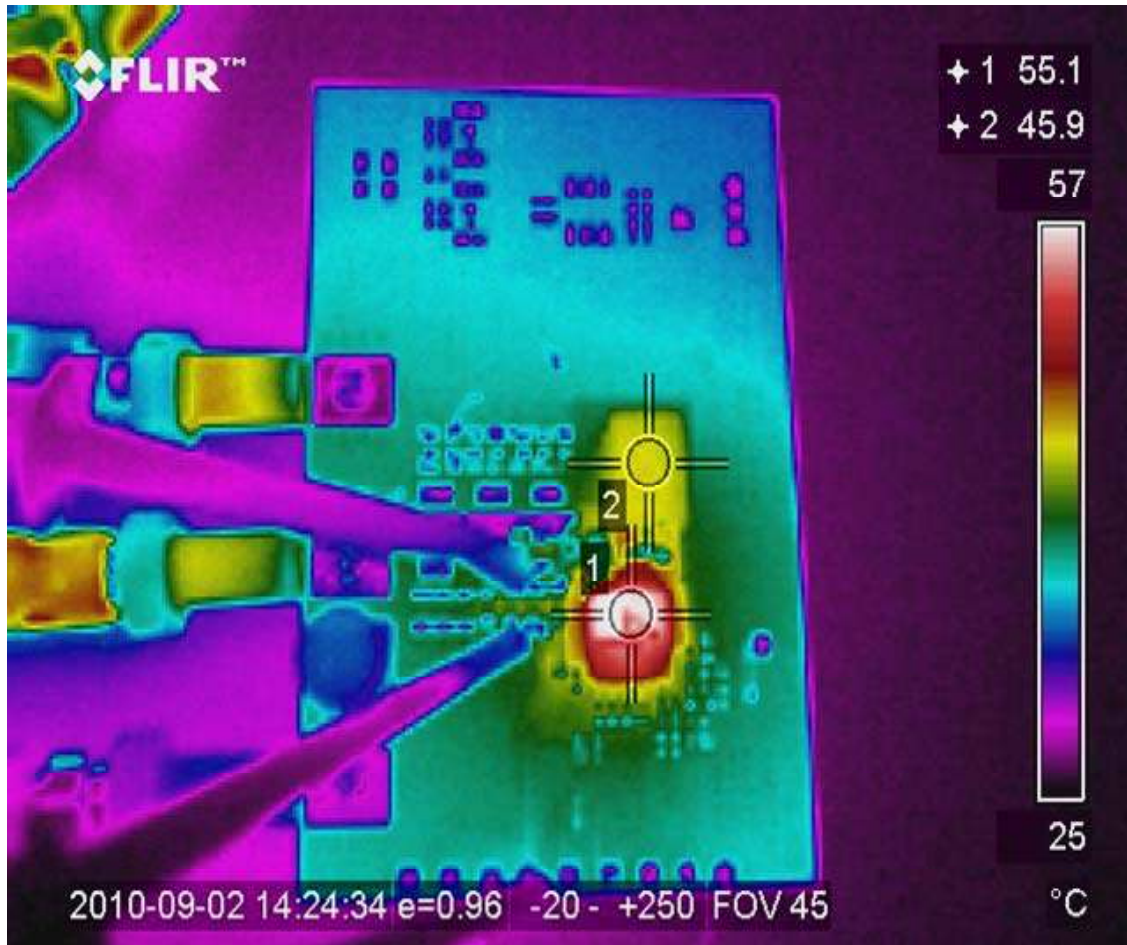
Figure 31: Thermal Image of the board at 25A load Test point 1 is iP1827 Test point 2 is inductor
