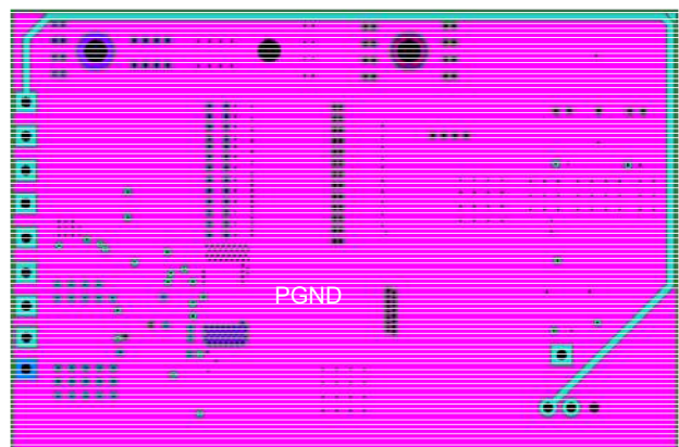
Figure 35f: IRDC1827 demoboard layout considerations – Mid Layer 4
