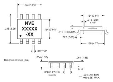
Note: SOIC8 Package has thermal power dissipation of 240°C/Watt in free air. Attaching the package to a circuit board improves thermal performance.
