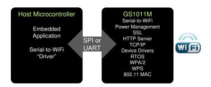
The GS1011M EVK Mrk II Evaluation Kit enables GainSpan customers to develop software on their existing microcontrollers to support the "AT" command set, and connect it to either the UART or SPI interface on the evaluation kit reference board.
