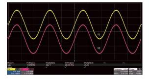
Output amplitude into a high impedance load can be as high 20 Vpp at frequencies up to 10 MHz, and 10 Vpp for frequencies greater than 20 MHz.
