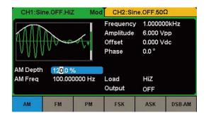
The T3AFG range of Function/Arbitrary Waveform Generators support a wide range of modulation types including AM, FM, PM, FSK, ASK, PSK and DSB-AM.
