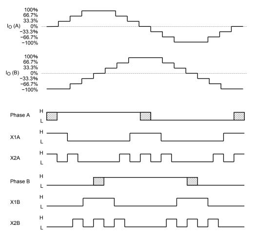
(\*) I<sub>O</sub>: OUT1 $\rightarrow$ OUT2; + current OUT2 $\rightarrow$ OUT1; - current
