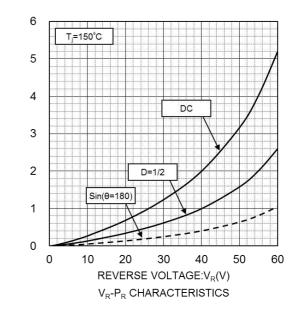
REVERSE POWER DISSIPATION:P<sub>R</sub>(mW)
