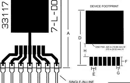
PINS ON .1 in. CENTERS PROVIDE COMPATIBILITY WITH BREADBOARDS AND SOCKETS.
