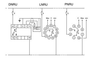
**Note:** The cable for probes (max 300ft) should be run in separate conduit. A shielded cable is recommended.
