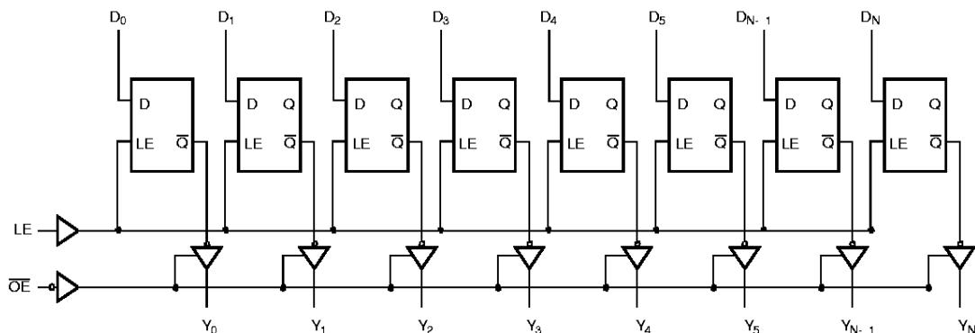
**Logic Block Diagram**
