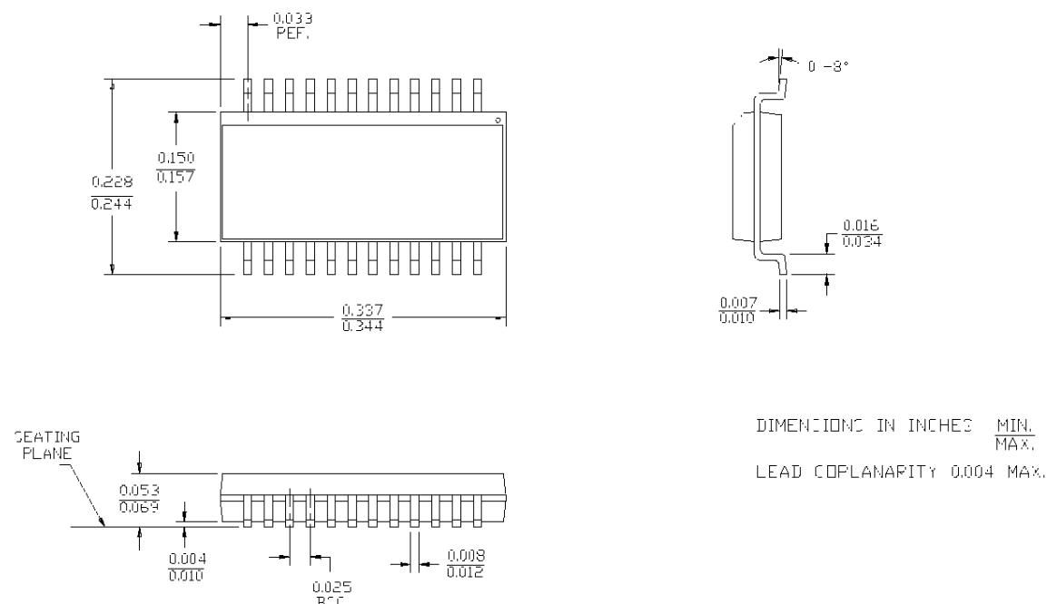
**24-Lead (300-Mil) Molded SOIC S13**
