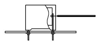
Temperature monitored inside the capacitor.
