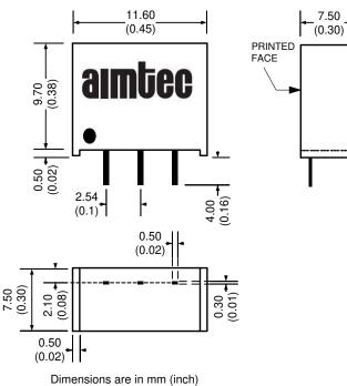
Pin Tolerance:  $\pm 0.16$  mm (0,004 inch) Case Tolerance:  $\pm 0.25$  mm (0.01 inch)
