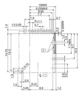
Note  $\bigcirc$   $\bigcirc$  indicates the center line of the microSD card slot.
