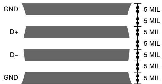
Figure 23. Typical Arrangement of Signal Tracks
